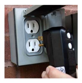
1. Plug the Ground Fault Circuit Interrupter (GFCI) into a working outlet.
